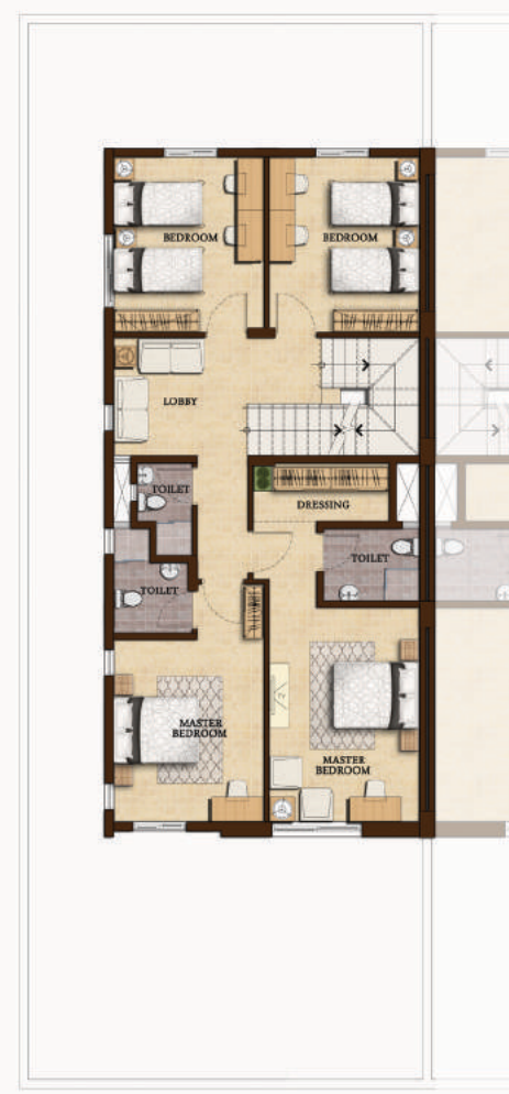
First Floor Plan Floor Area - 120.80m 2
